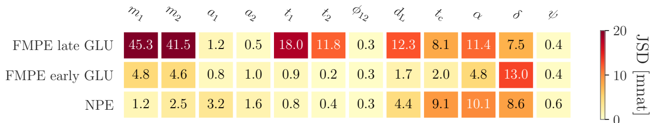
Figure 3. Jensen-Shannon divergence between inferred posteriors and the reference posteriors for GW150914 (Abbott et al., 2016). We compare two FMPE models with the same architecture as the NPE embedding network, see Tab. 1 bottom panel. For the model in the first row, the GLU conditioning of (\theta, t) is only applied before the final 128-dim blocks. The model in the middle row is given the context after the very first 2048 block.
